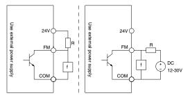
Figure 4-9 FM terminal wiring
