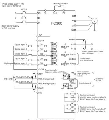
Figure 4-5 FC300 control terminal wiring diagram
