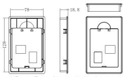
Figure 8-1 The size of the external lead installation base
