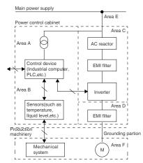
**Area A:**Control power transformer,control device,sensor,etc.
