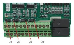
Figure 4-1 Jumper position (0.4~37kW)
