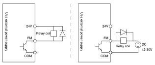
Figure 4-8 FM terminal wiring
