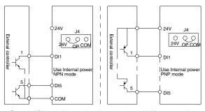
Figure 4-6 DI terminal input wiring when using internal 24V power supply
