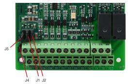
Figure 4-2 Jumper position (45~400kW)
